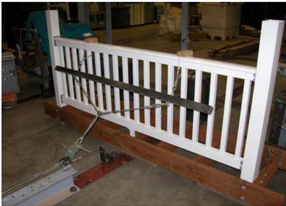
Figure 3. Uniform load test setup
