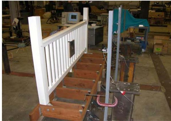
Figure 2. Guardrail setup for the in-fill test
