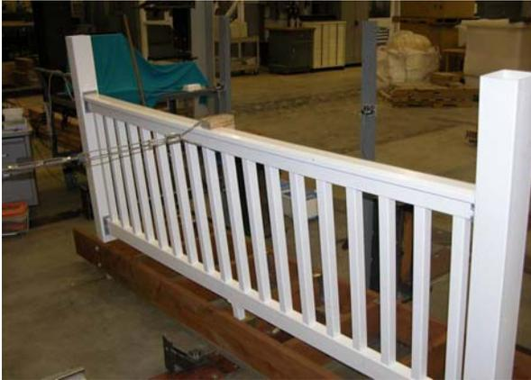
Figure 4. Concentrated top rail load test
