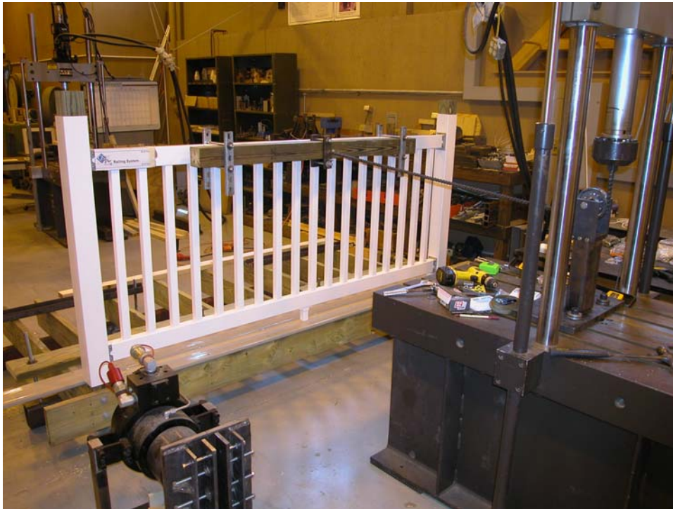
Photo 1: Test set-up showing rail system and test machine.
